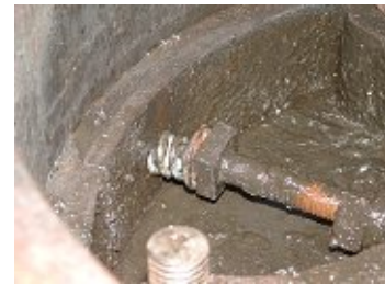
Inside of piston showing one spring on end of adjusting screw (10)
