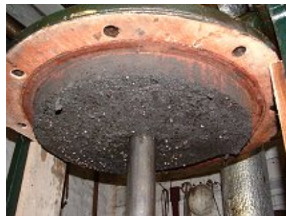
Underside of piston showing contamination (5)
