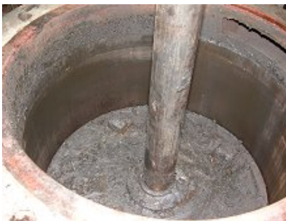
Top of piston showing contamination (5)
