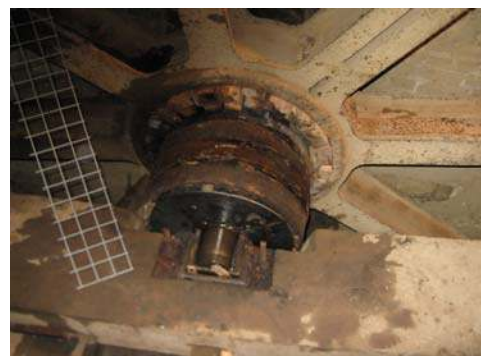
Metal disc screwed to end of shaft to retain wedges
