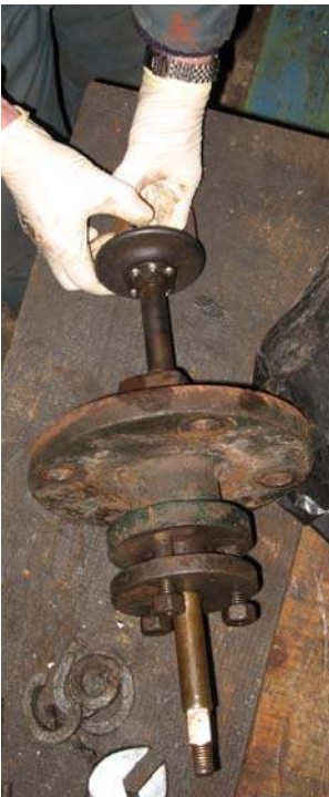
Valve top, spindle and cone after repair
