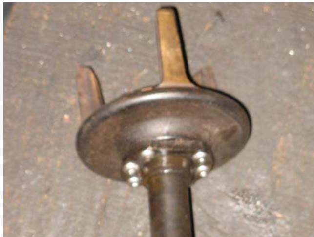
Close-up of cone showing the repair with stainless steel screws
