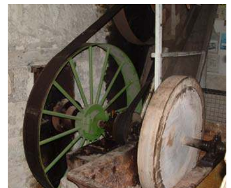
Plinth, bearing, coupling, whet stone and belts fitted and ready to run
