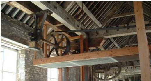
Lay shaft taking drive from line shaft to lathe and bandsaw
