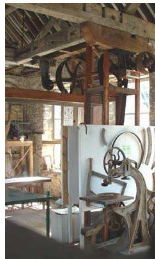
Bandsaw below lay shaft
