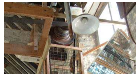
Striking gear for lathe to enable it to be started and stopped
