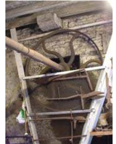
Pulley on line shaft to drive forge fan
