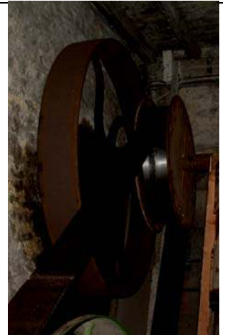
The new 24" dia pulley with flanges alongside the original pulley drive from the engine
