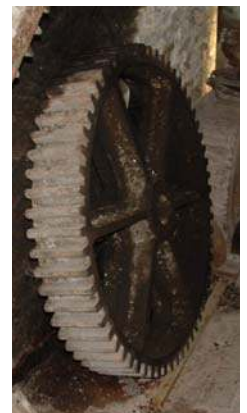
Gear wheel which drives line shaft. Now on floor
